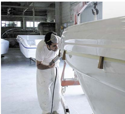
Fig. 8 Sealing with Sikaflex®-295 UV
