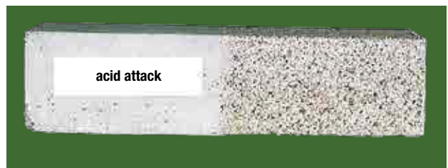
Acidic attacks which dissolve calcium compounds out of the hardened cement matrix can be caused by acids, exchangeable salts, vegetable and animal fats or oils. Degradation of the concrete usually occurs very slowly. (Picture: BetonSuisse, Merkblatt 01)
