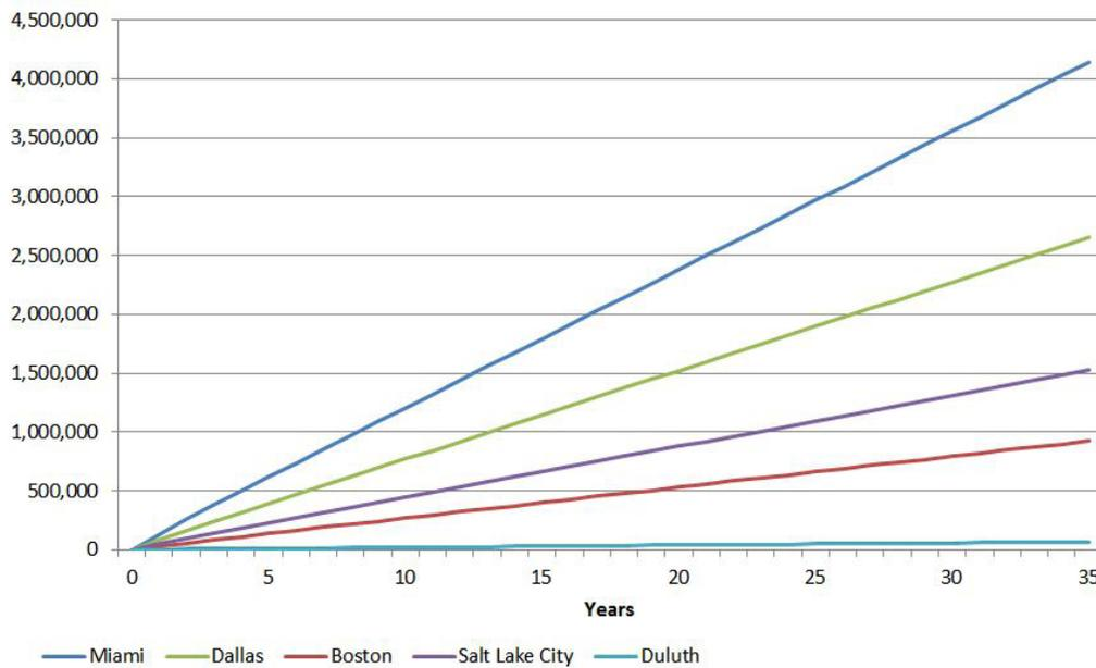
**Estimated cumulative potential greenhouse gas emissions savings due to the use of a white Sarnafil S 327 membrane compared with a black roof:
