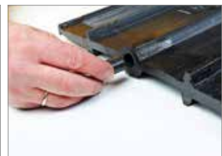
Plugging of the centre bulb with a cellular foam plug and inserting a raw rubber plug
