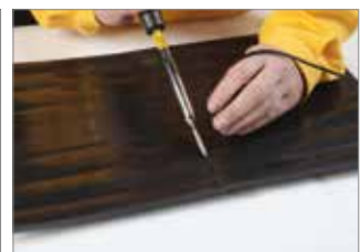
Strengthening with welding strip using welding tip
