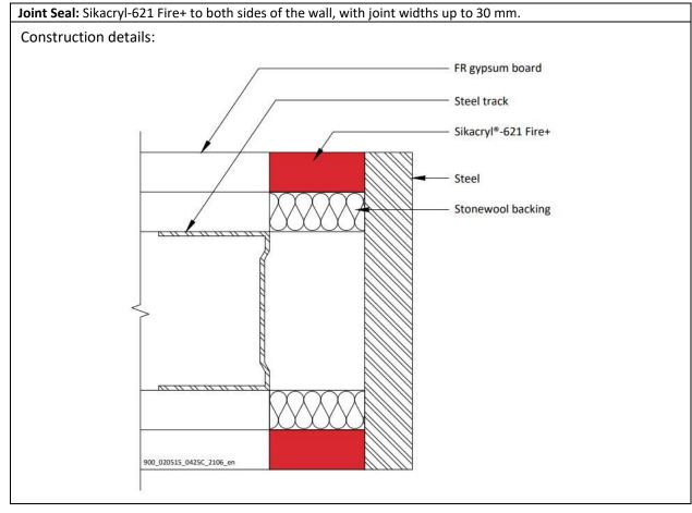
A.2.5 Linear joint or gap seals, vertically or horizontal orientated with backing materials
